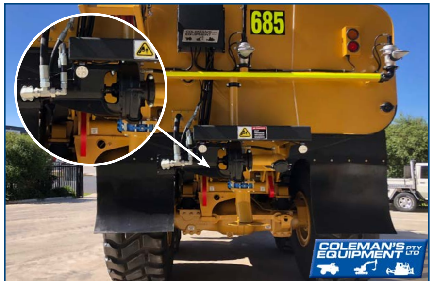
101-B73403GR shown here on Coleman's Equipment 8,000 Gallon CAT 745 Tank System.
