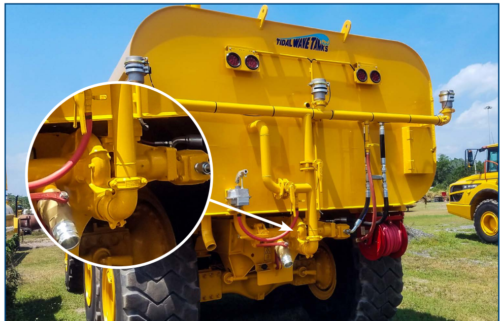
101-B69875 Pump shown here on an 8,000 Gallon, Volvo A40G Tank System Manufactured by Tidal Wave Tanks, Mulberry Florida
